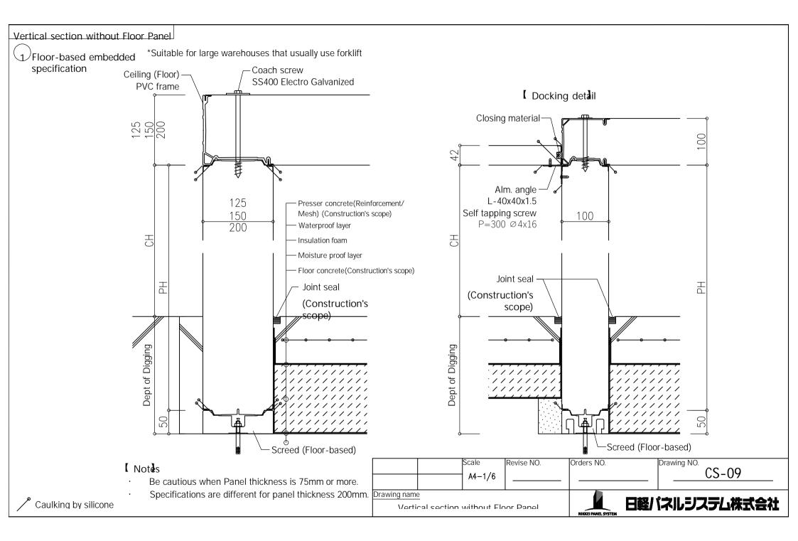
Vertical section detail at Floor without Floor Panel 1 \*Please determine the specifications according to the intended use
